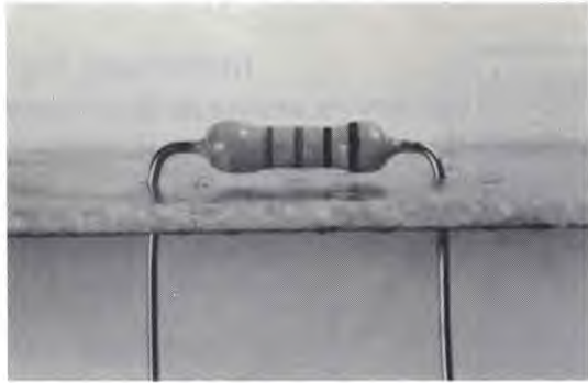
Figure 3: This resistor is partially inserted – the body will finally touch the top of the PC board and the leads on the copper side bent to retain the resistor in position prior to soldering.
